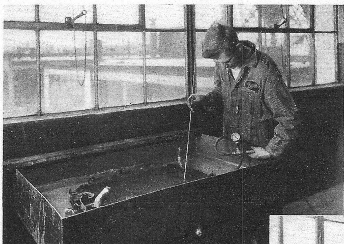
Locating leaks by using air at low pressure on radiator which is immersed in a tank of water.
