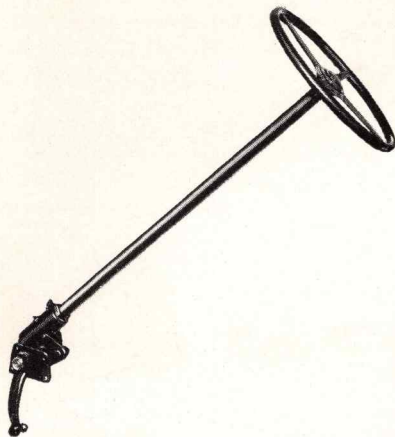
Improved worm and sector type steering system, with increased gear ratio
